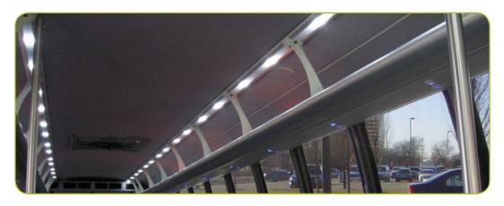
Swan systems provide a motorcoach experience for shuttles with reading lights and air conditioning vents for personal comfort.
