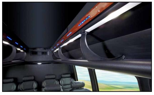
Complete interior system customized to fit your needs. The base luggage rack is window to window modular in length utilizing the overhead Omega light channel. This simple and durable luggage rack has different options of storage floor. Optional amenities make the Xtreme Interior System fully upgradable with reading lights and night lights.
