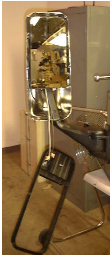
Image 1 (left) – Bezel removed and hanging from heater wires
