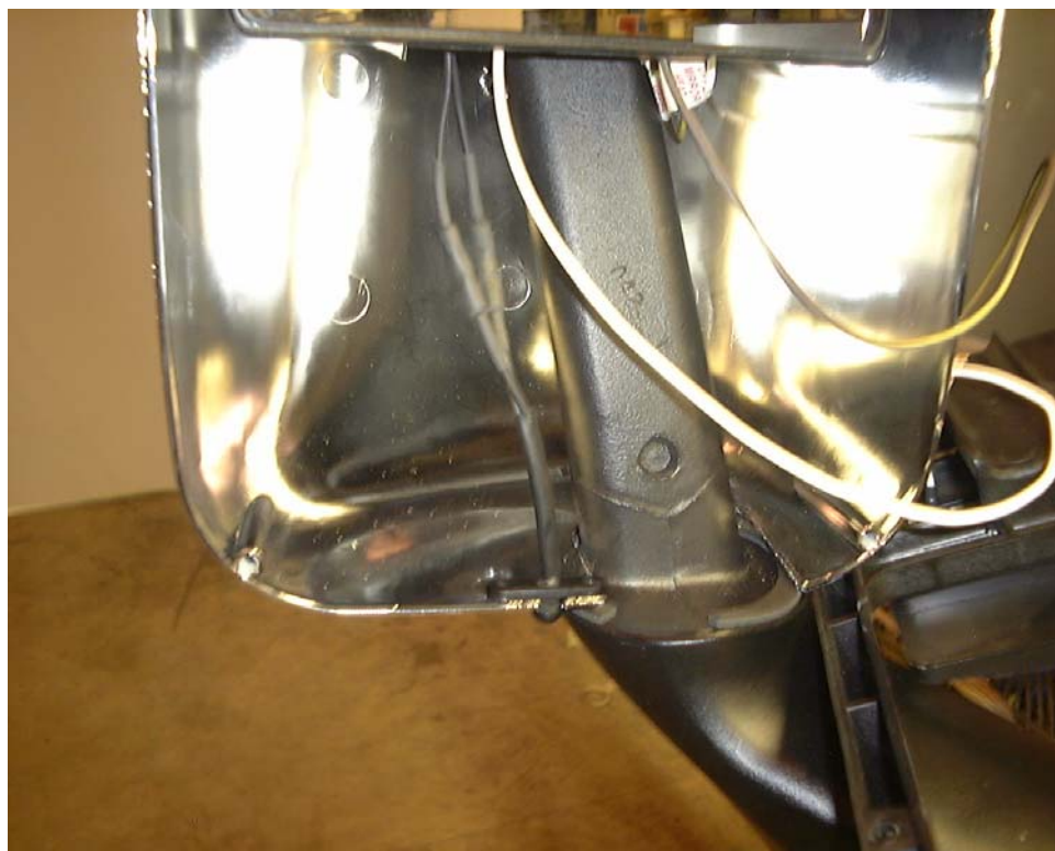
Image 5 – Splice connections covered with heat shrink tubing, and new sensor placed into slot on mirror shell
