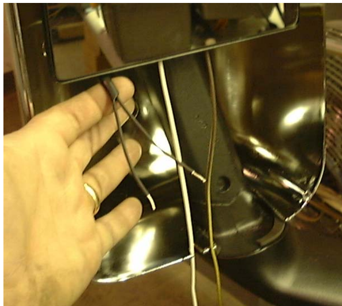
Image 3 - View of sensor harness after removal of defective sensor
