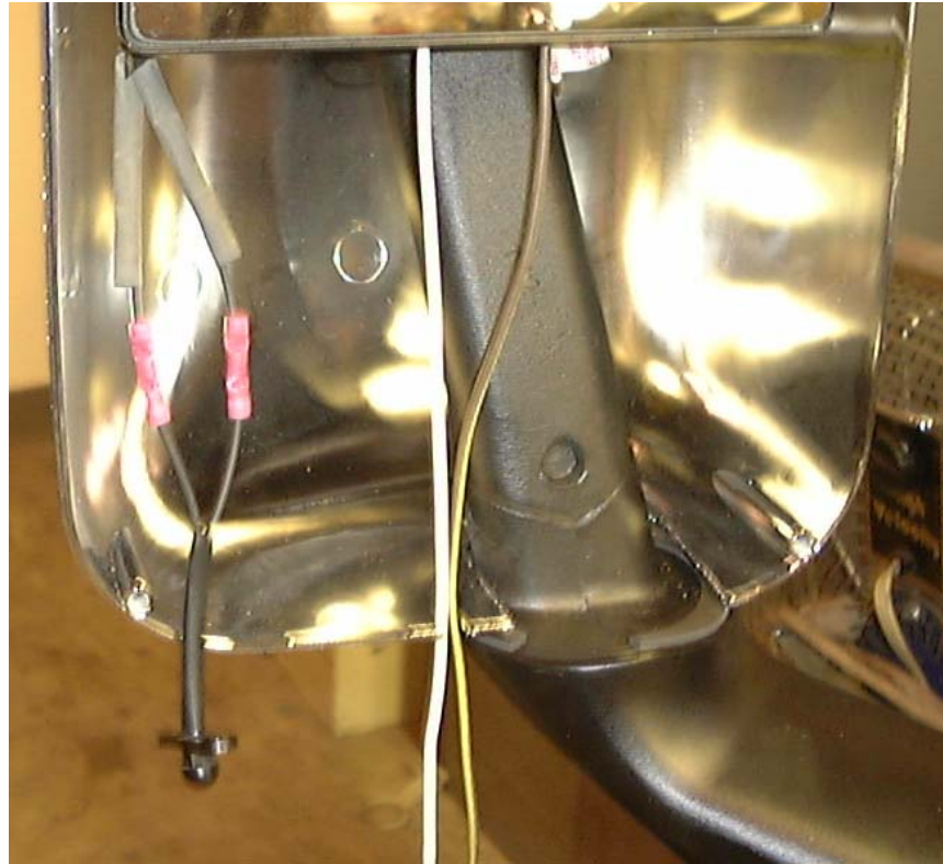
Image 4 – New sensor connected to existing sensor harness with the use of butt splices
