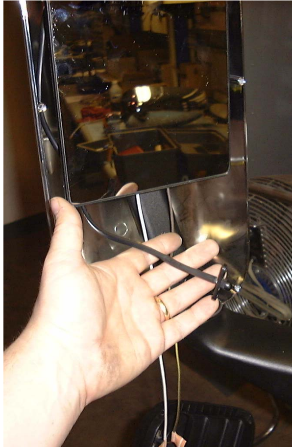
Image 2 (right) – Sensor exposed after removal of bezel
